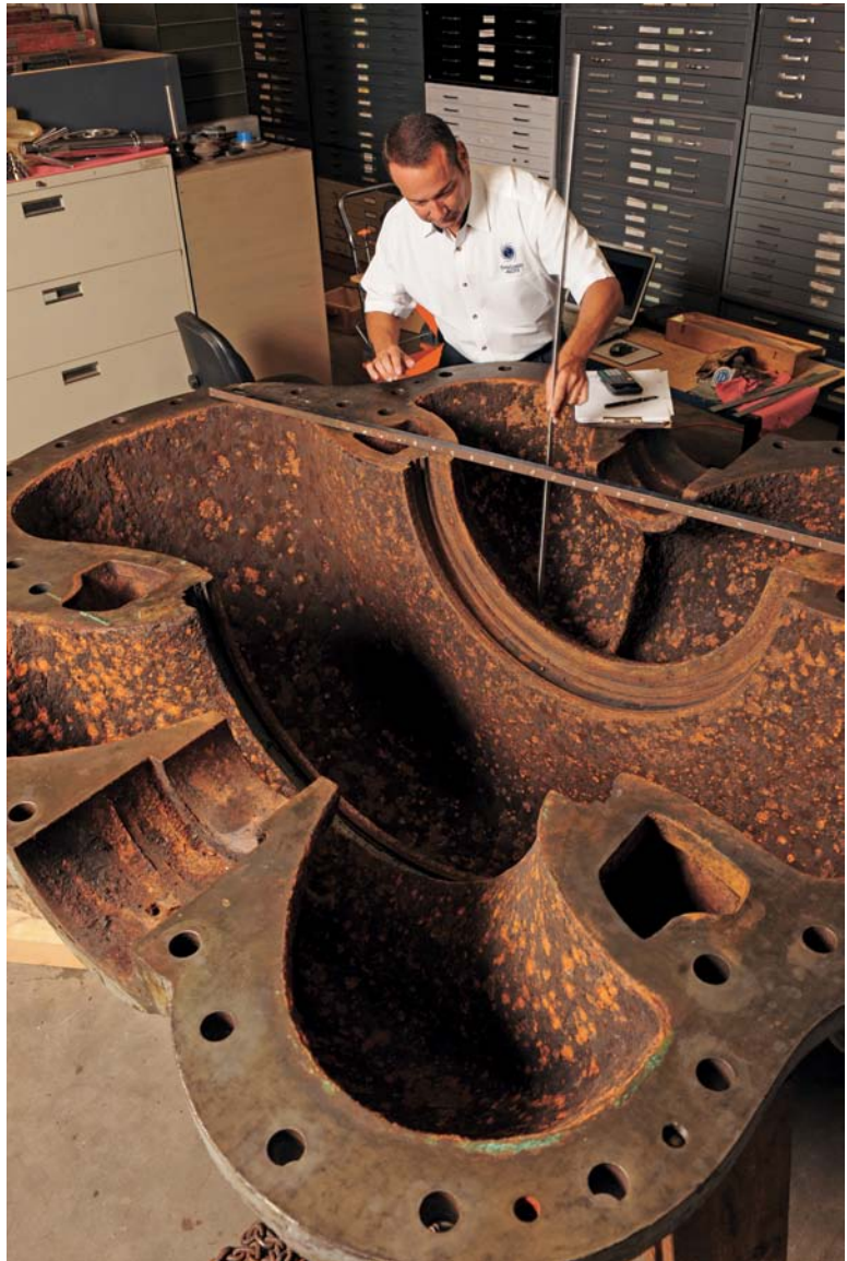
Reverse engineering a pump case
