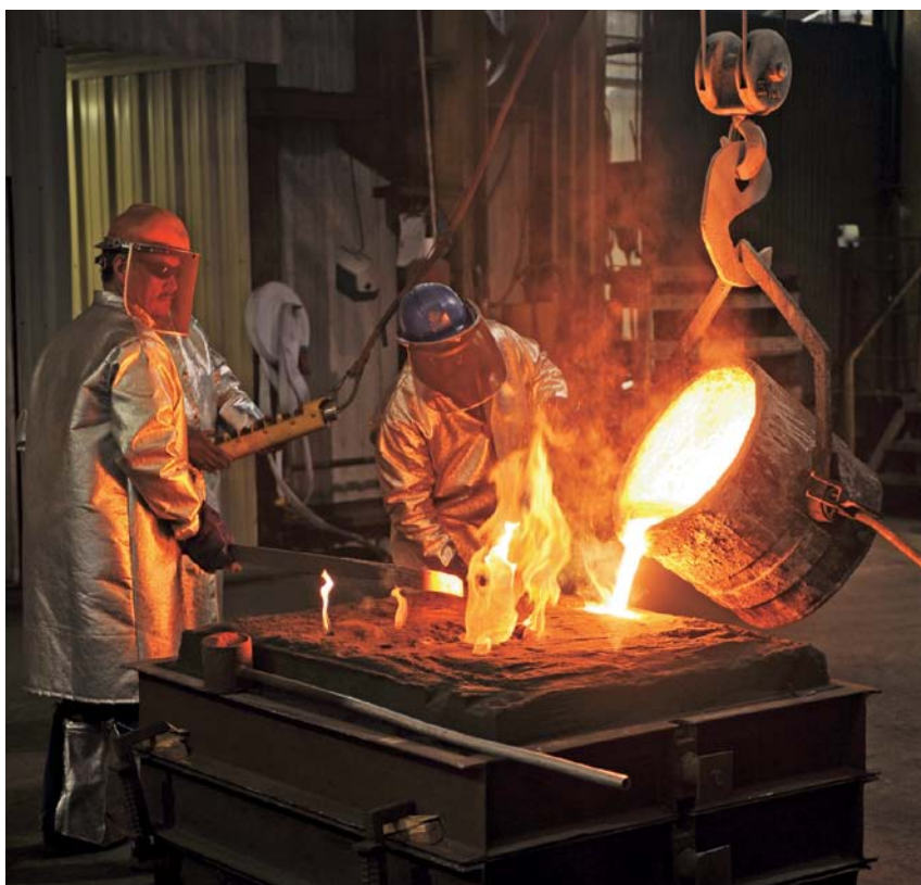
Pouring metal into a mold
