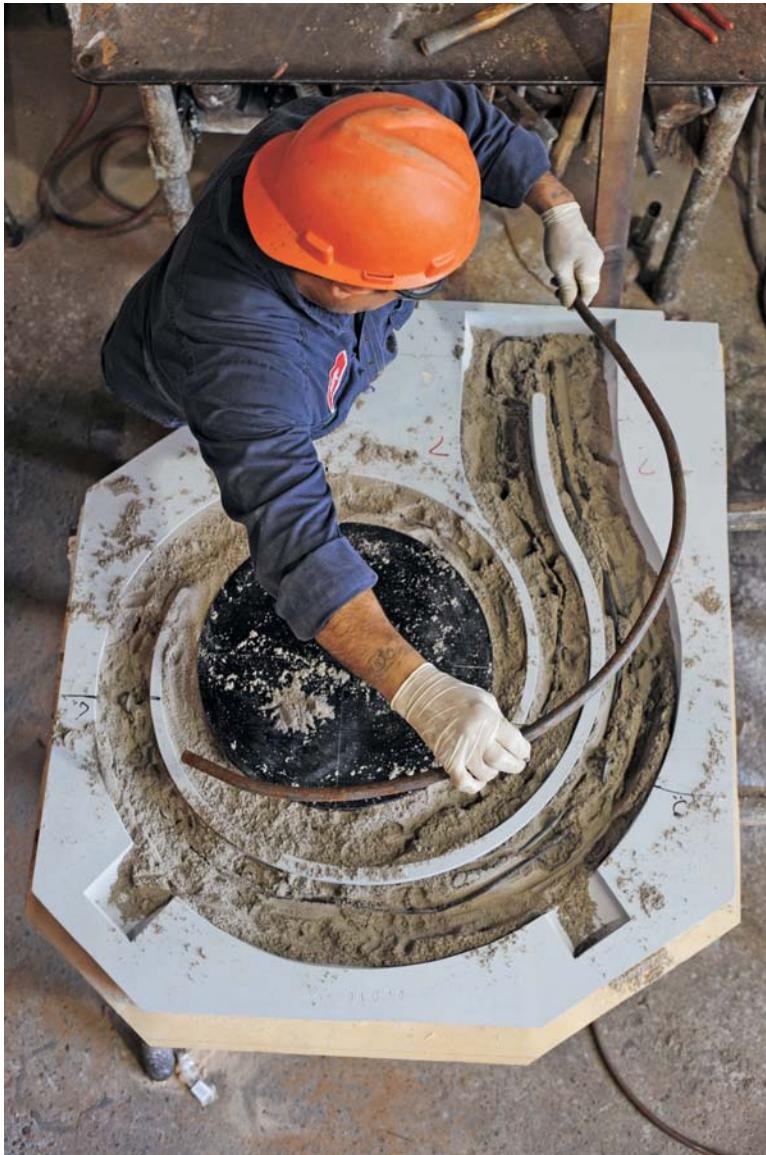
Making a sand core in a core box
